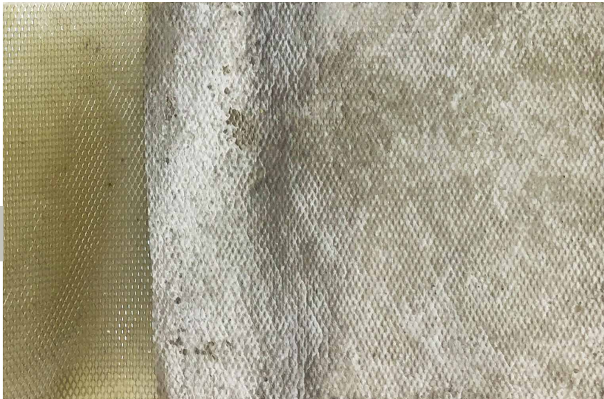
Wire mesh coated in liquid latex, then dipped in concrete.
