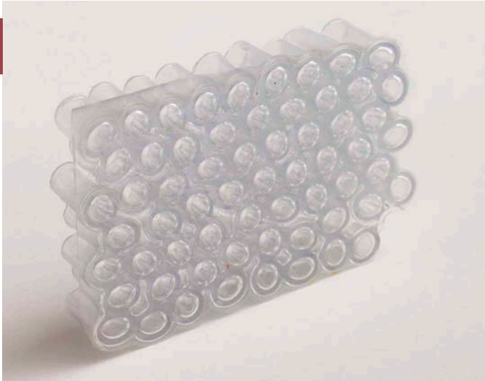
Test with creating cell structure by connecting pieces of PVC tubes using resin
