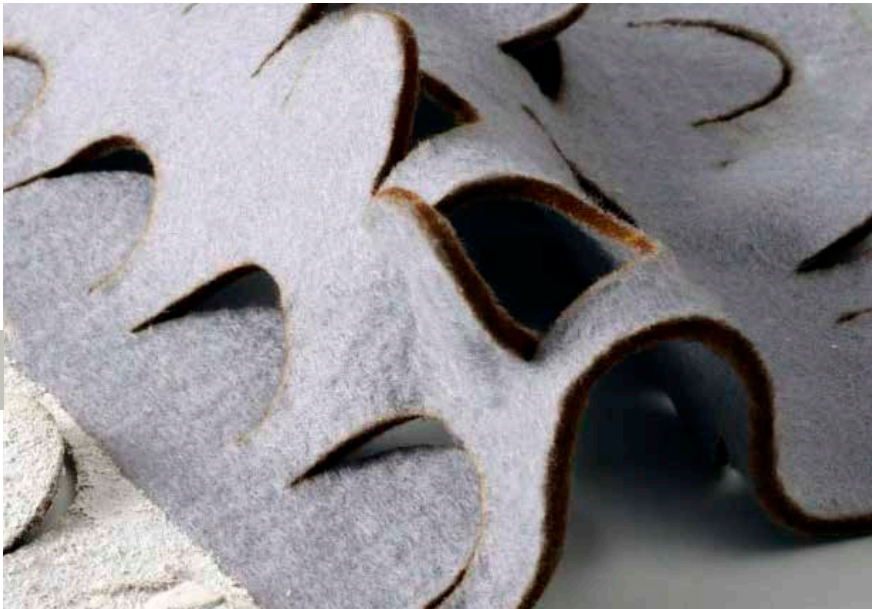
Laser Test: 2 mm felt laser cut and then partly dipped into plaster.
