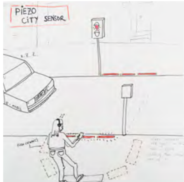
9 sensor integrated in the pavement
