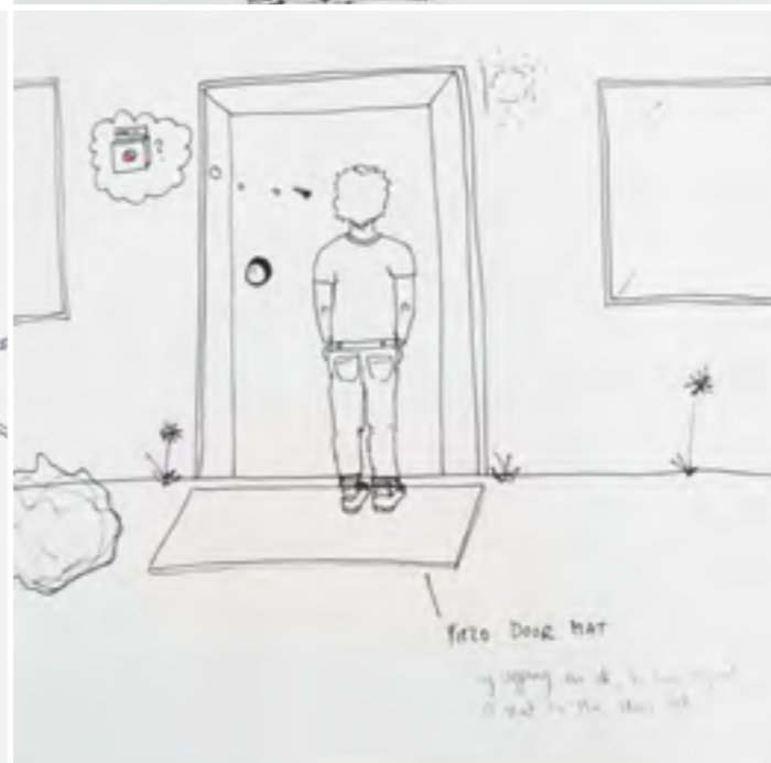
10 the PIEZO senses the presence of a person
