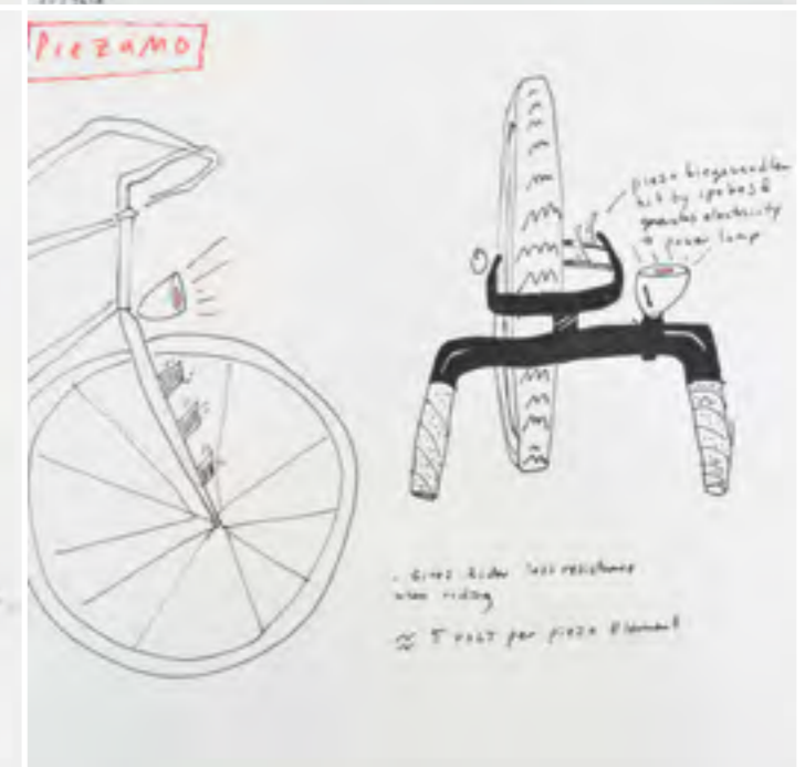
14 PIEZO generator to substitute a regular dynamo
