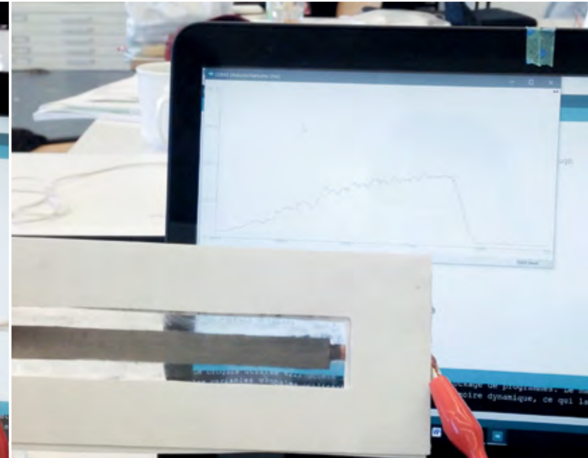
19 sensor being deformed with less pressure
