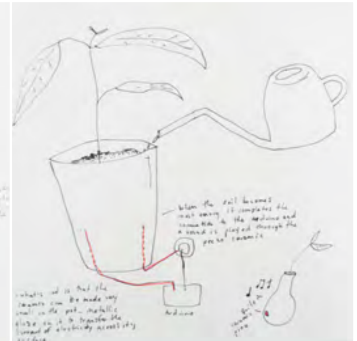
12 PIEZO making sound when plant needs water
