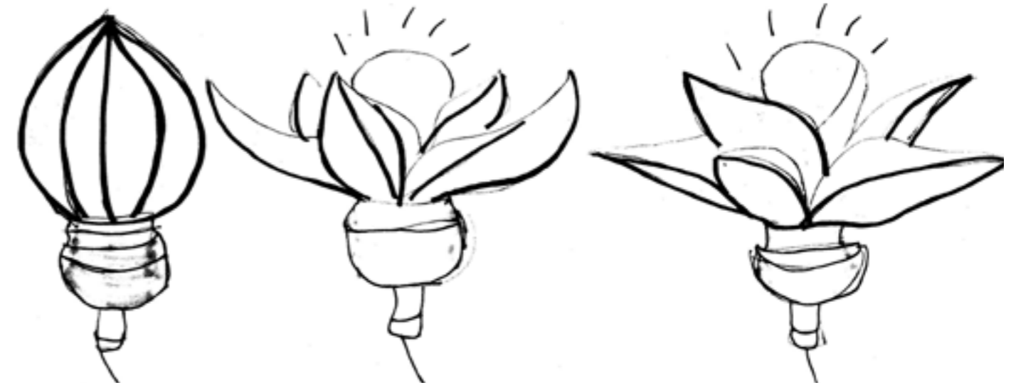
22 using the shape changing effect of EAP to open and close a surface
