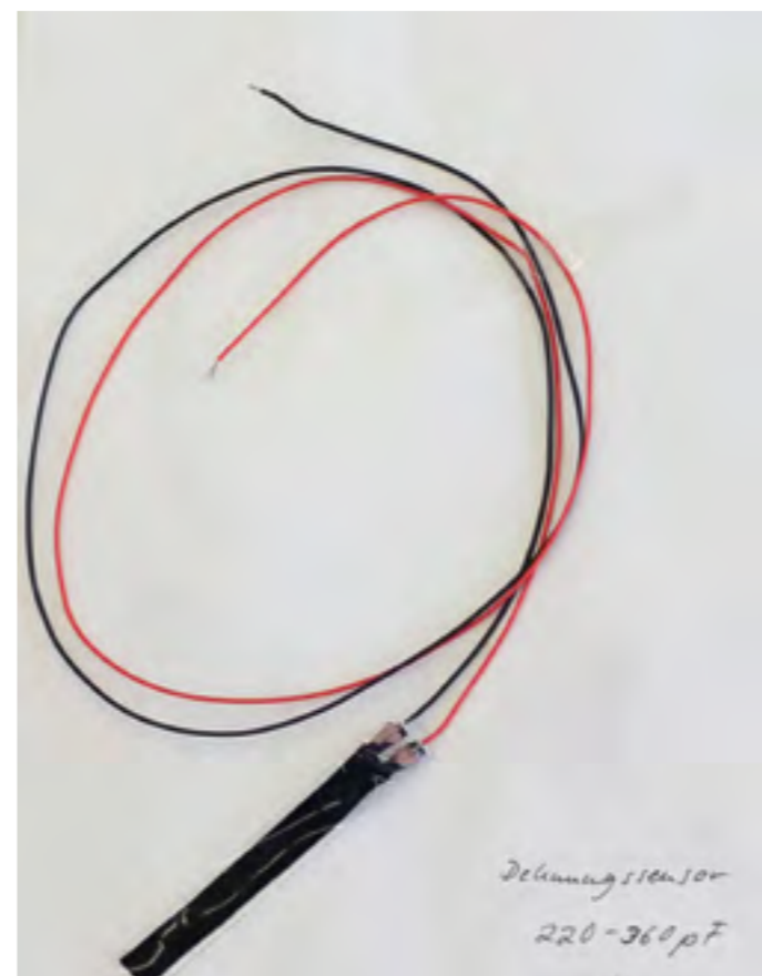
15 lab-made stretch sensor by Fraunhofer CesMa
