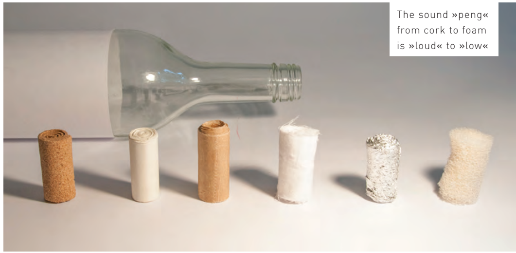
Experiments with plugs in a row from »hard« to »soft«, paper, cork, baking paper, aluminium, foam
