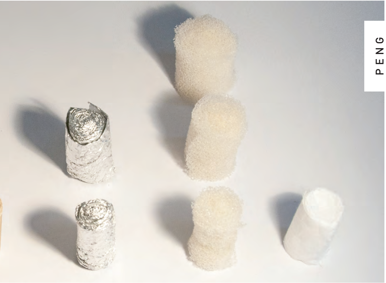
Experiments with plugs in a row from »hard« to »soft«, paper, cork, baking paper, aluminium, foam
